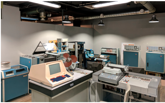
1. Room dedicated to the Elwro Odra 1305 Computer from the 1970s; two square objects on the right are the central units: equivalents of contemporary microprocessors
