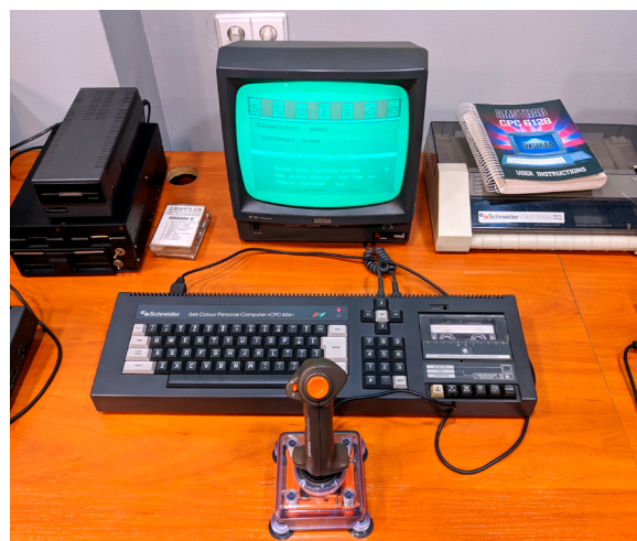
3. An example of a highly authentic interaction spot: Amstrad/Schneider CPC 464 home computer (produced from 1984) with a monochromatic GT 65 screen, DMP3000 dot matrix printer, 3 inch FDD, and a set of pirated games on tapes; instruction in English relevant for CPC 6128
